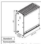
(pluggable module for 19" sub-rack) approx. 5.0 kg \*) applicable to 5 V output models
