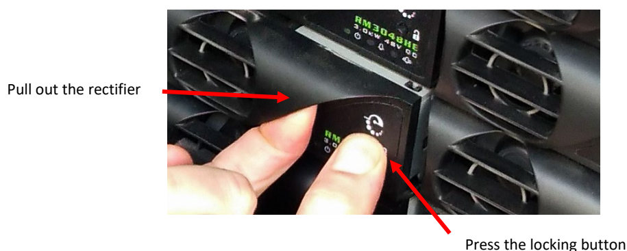
Figure 20: Removing a Rectifier
