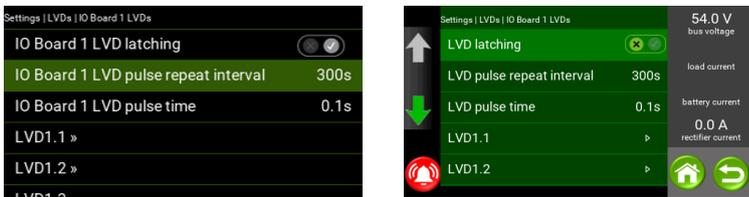
The EM4x can control up to 2 magnetically latched contactors. It can control up to 3 Normally Open or Normally Closed LVD contactors. Magnetically latched contactors require no energy to keep them closed or open, only a pulse to make them change state, whereas N.O. or N.C. contactors require permanent energy to keep them in one state or the other.
