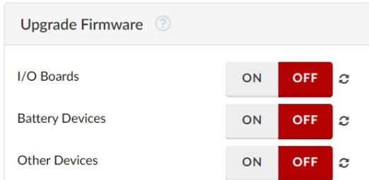
**NOTE:** as of ena firmware release 7.0 **Battery Devices** includes energypak only and there are no **Other Devices** that auto-upgrade firmware.
