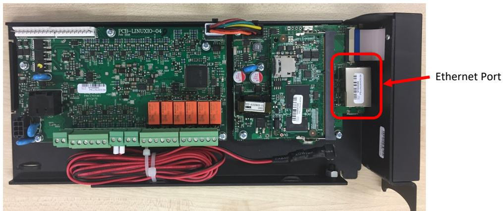
1. Connect the communicating device to the J305 Ethernet port inside the energy manager.
