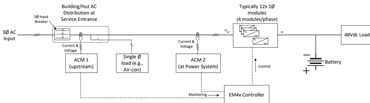
As shown, two Enatel AC Monitors (ACMs) are required, with current transformers at each monitoring point.
