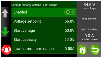
**Fast Charge Voltage Setpoint** is the target bus voltage that the EM4x tells the rectifiers to aim for during the Charge session. Set this value to that recommended by the battery manufacturer (usually between 2.3V/cell to 2.4V/cell (55.2 and 57.6 for 48V systems) at 25°C). Note that this voltage is temperature compensated.
