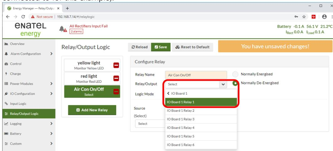
4. Select the **Normally De-Energised** or **Normally Energised** radio button as required.
