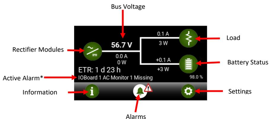
\*NOTE: when there are multiple alarms raised the Active Alarm display cycles through the list. The complete list can be viewed in the Alarms menu.
