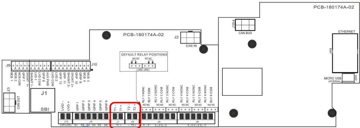
Figure 15: EM4x Relay State Jumpers
