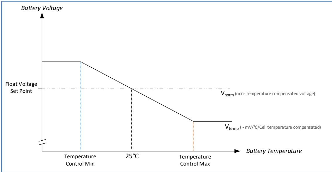
Figure 22 shows the temperature compensation function varies the float voltage of the system based on the float voltage set point, the slope and the measured battery temperature.
