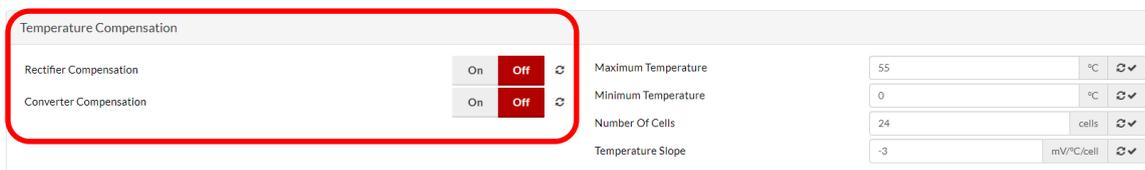
From the front panel interface navigate to Settings>Temperature compensation>Enabled (rectifiers)
