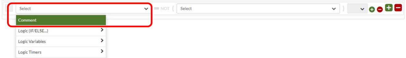
Selecting **Comment** allows descriptive text to be entered to provide insight as to the function of sections of the input logic.
