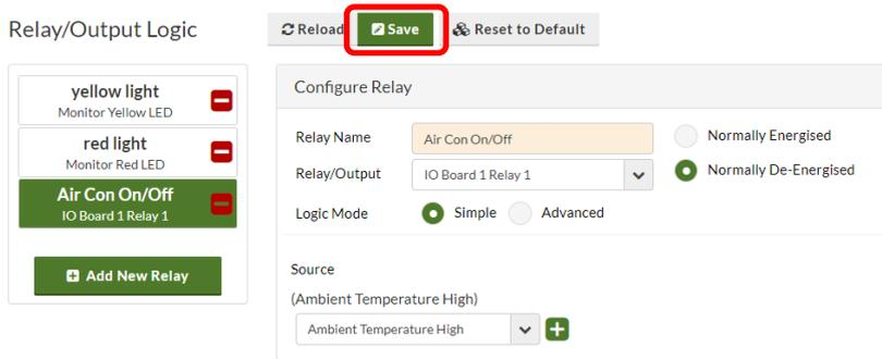
*Comment:* example 1 is now complete. As the Ambient Temperature High alarm triggers or de-activates the relay energizes or de-energizes to turn the air-conditioner on and off. Note however in actual application further conditions would usually be applied to this function.
