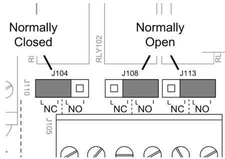
Relay 1 is permanently configured as Monitor OK, and as such is in a Normally Energised state.
