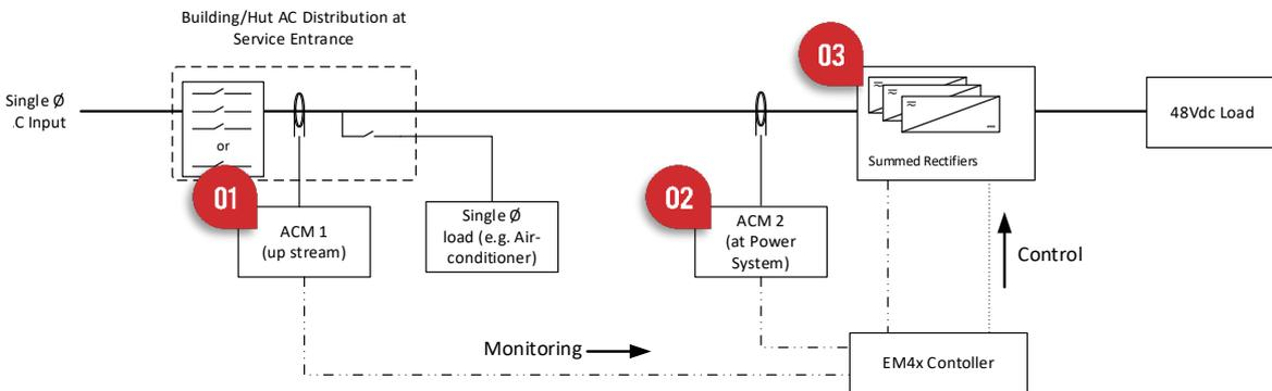
In Figure 24 an AC Monitor at location 01 would be used to protect breakers in the distribution board. Either an AC Monitor at location 02 or the summed rectifier currents at 03 could be used to protect breakers in the power system.
