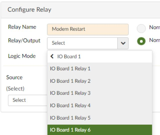
5. Select **Ping Failed Critical** from the **Source** drop down menu: Alarms>ICMP>Ping Failed Critical.
