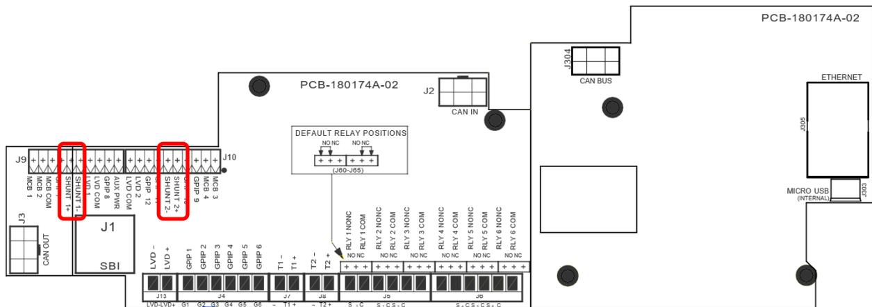
The current sensors must be placed in the negative of the DC system. When the current sensors are wired to a controller, a 4k7 resistor should be placed in series with each sense wire at source. The main reason for this is to protect the sense wire, however, it also provides the required input resistance to a controller to maintain the calibration. Current shunts are available from Enatel which already have these resistors fitted.
