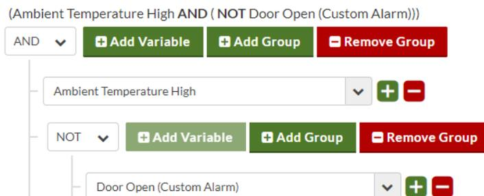
*Comment:* the examples are now complete. The air conditioner turns on at a particular temperature and off at another. There is a door open alarm which turns on a light when the door opens and turns the air-conditioner off when the door is opened.
