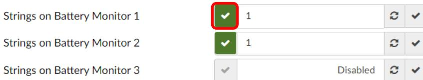
Enter the number of strings of batteries connected to the battery monitor.
