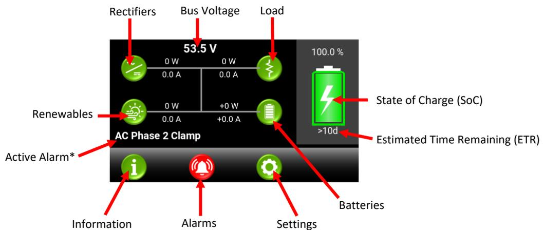
\***NOTE:** when there are multiple alarms raised the Active Alarm display cycles through the list. The complete list can be viewed by tapping Alarms.
