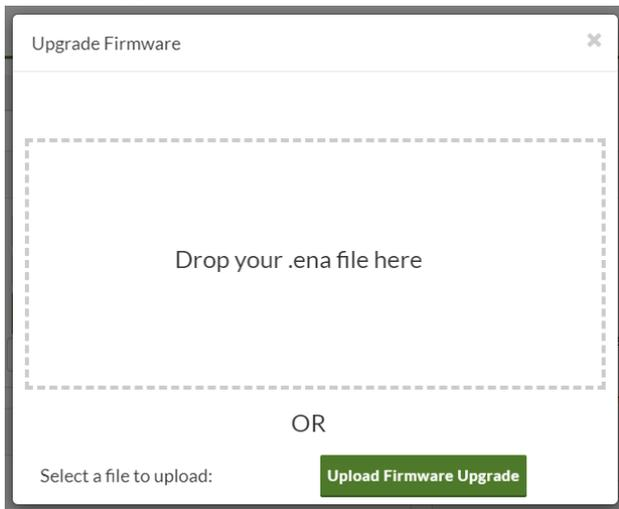
5. The firmware upgrade automatically completes for the EM4x and those ancillary devices enabled. During the process the EM4x reboots and as the final action the Web UI reloads.
