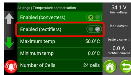
To set the **Maximum Temperature**, **Minimum Temperature** and **Temperature Slope** consult the relevant battery specifications.
