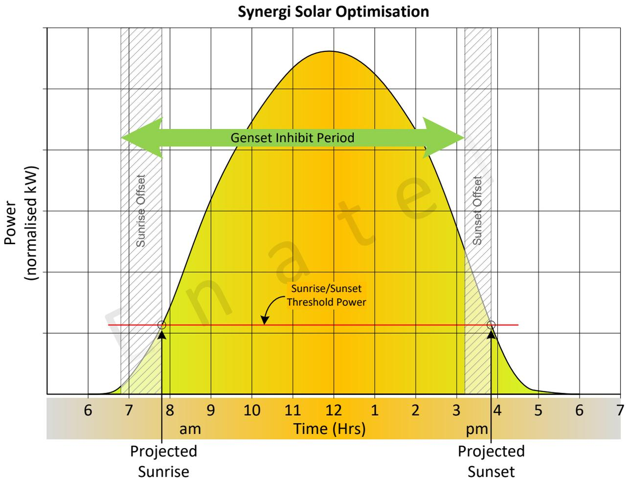
As shown in Figure 27, SYNERGi creates a Genset Inhibit Period. This includes offsets to optimize the period the generator should run.
