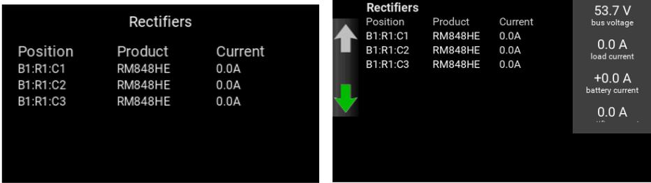
Selecting an individual rectifier displays the serial number, the firmware number, the active current and any alarms raised.
