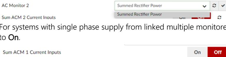
For systems with single phase supply from linked multiple monitored cables toggle the **Sum ACM Current Inputs** to **On**.
