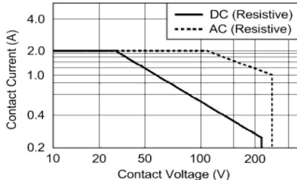
**NOTE:** The relays fitted are not suitable for use with inductive type loads. A suitably rated interface relay should be used for inductive load applications.
