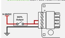
Example: DOTL alarm, Red LED and Sounder activated together from one output.
